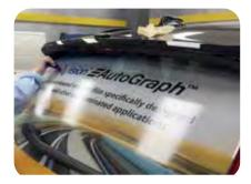
Contra Vision® AutoGraph™ one-way vision graphics is specifically designed for vehicle windows. It is highly conformable and features air release channels within the adhesive so when overlaminated and applied to glass, any trapped air can escape resulting in a smooth and bubble-free application.
